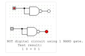
(2) p D ~p = T p D ( p D p ) Applied Propositional Logic: theory, simulation code, and digital circui...
