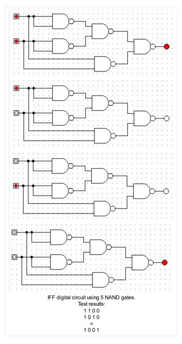
What might these circuits be used for? NOT, AND, OR have clear applications when combining signals. XOR and IFF are useful for various signal comparison (distinct or same). TRUE/FALSE are useful when one needs to maintain steady signal regardless of the variation. An example applications for IMPLY is to detect cases when the implication fails, e.g. NOT-IMPLY, as this will alarm (signal high) when p=1 but q=0, while all other cases will output signal low.
