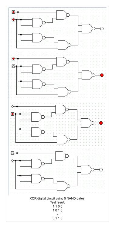
(9) ( ~p D ~q ) D (p D q) = p <-> q p dup D q dup D D p q D D .. = 1 0 0 1 b 5 NAND gates
